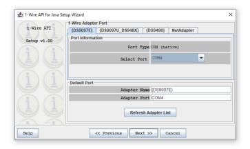
If you see a message box with error message 1-Wire Net not available, it means 1-wire device has not been detected. This is usually caused by selecting wrong Port.
