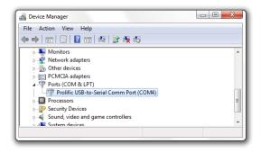
This name COMx with corresponding number x represents connected device.
